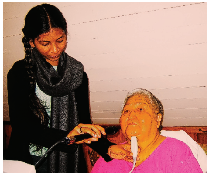
Fig. 2. Data collection from speaker Margery Inkster with a portable ultrasound machine. The probe is held under the chin, giving a view across the tongue.
