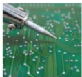
When two objects are in direct physical contact, such as the soldering iron and the circuit board, heat is transferred by conduction . Energy is transferred by direct contact.
