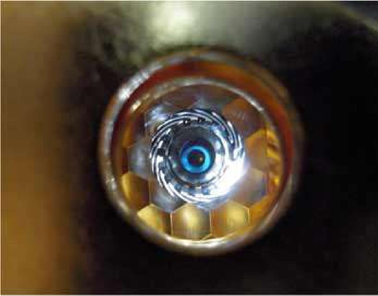
A view of a cryogenically cooled NIF target as "seen" by the laser through the hohlraum's laser entrance hole. In ignition experiments, the hydrogen in the fuel capsule must be compressed to about 100 times the density of lead.
