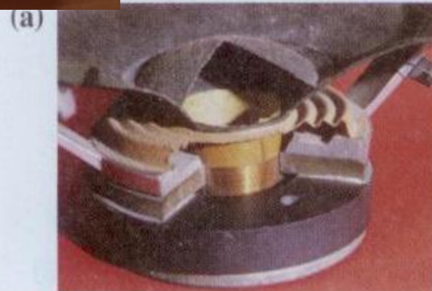
24.61 The arrangement of the coil and magnet poles in a speaker.
