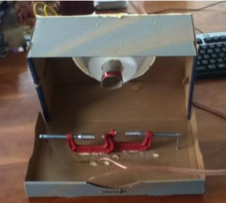
24.61 The arrangement of the coil and magnet poles in a speaker.
