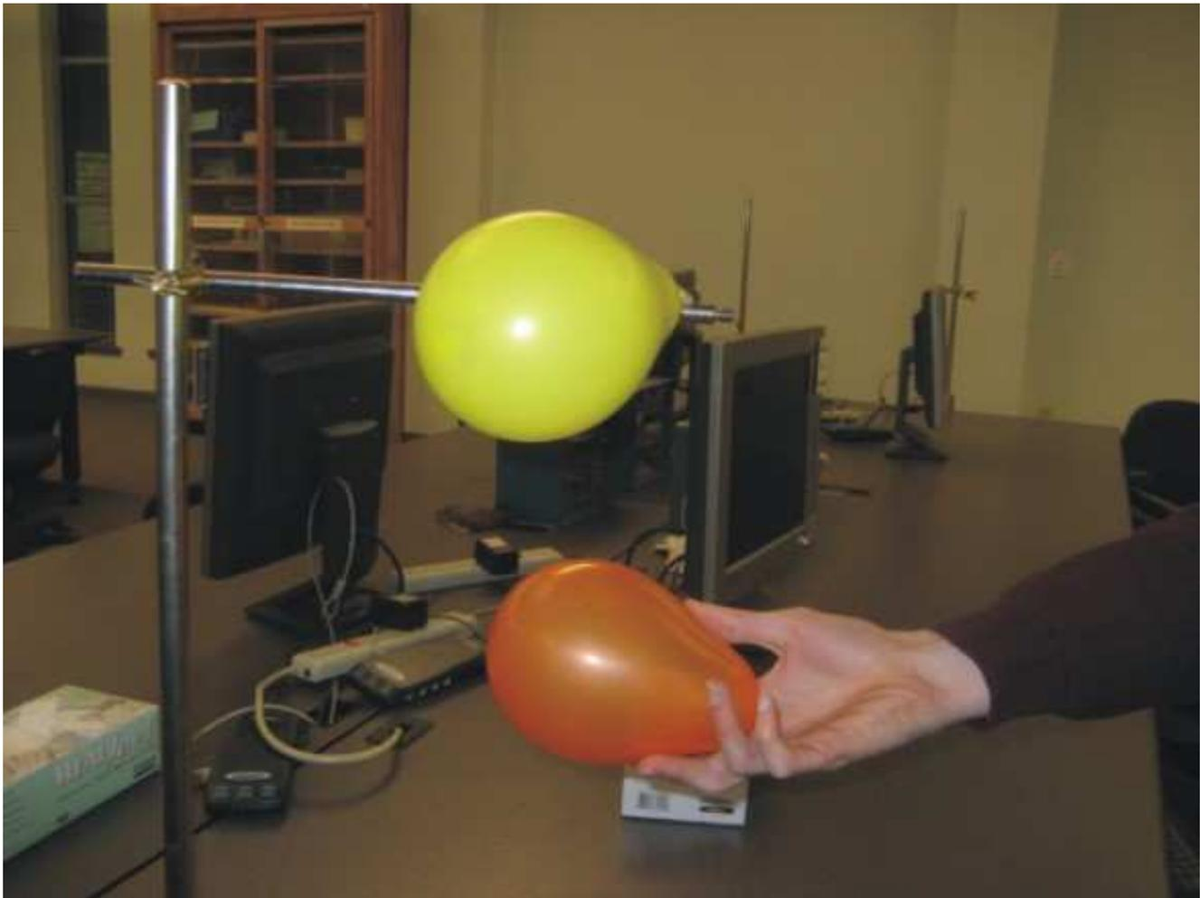
8. Quickly estimate or measure the distance from the bottom of balloon 1 to the top of balloon 2. Record this measurement  $D$  and your estimate of the uncertainty of this measurement in the spreadsheet.
