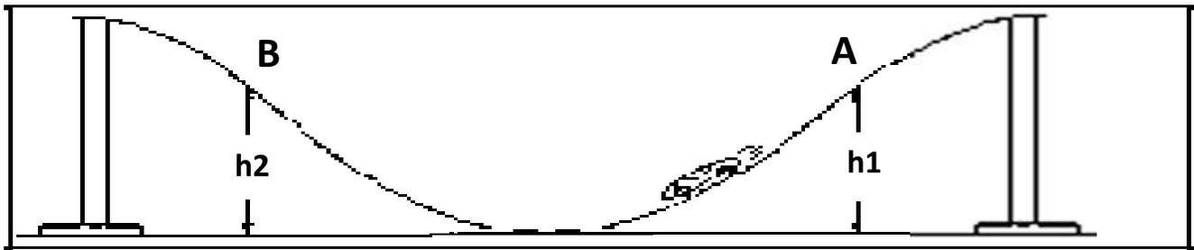
Release the car from the starting point A. Record this height ( $h_1$ ) and the height to which the car rises ( $h_2$ ) on the other end of the track. Complete several trials. It is important to secure the track to the floor so some of the car's energy is not transformed into motion of the track.
